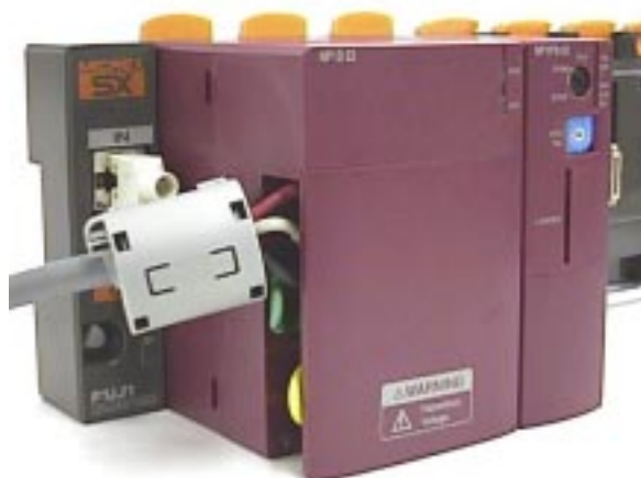
Wire to a power supply and grounding wire
