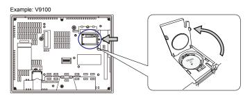
Insert a precision screwdriver into the gap on the right side of the battery and lift the battery out.
