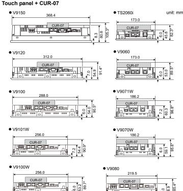
Including the screw connector supplied with CUR-07
