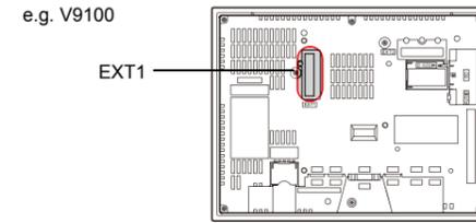
2. Align the three mounting screw holes on the CUR-04 with the holes on the V9 series or TS2060i, and lightly press section "A" of the CUR-04. Check if the unit fits in the connector.
