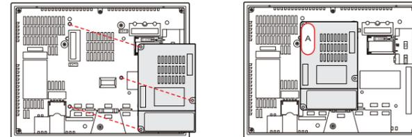
3. Fix the CUR-04 on the V9 series or TS2060i using the three mounting screws supplied with the CUR-04. Also, connect the CUR-04 (the metal in the lower left) and the V9 series or TS2060i frame ground (FG) using the provided FG wire.
