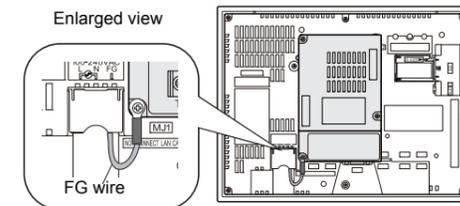
\* In the case of TS2060i, connect the provided FG wire to the FG terminal for communication on TS2060i.
