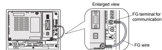
4. Wire the communication cable. For more information about the communication cable, refer to "Specifications of Communication Unit PROFIBUS-DP."
