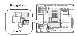
\* In the case of TS2060i, connect the provided FG wire to the FG terminal for communication on TS2060i
