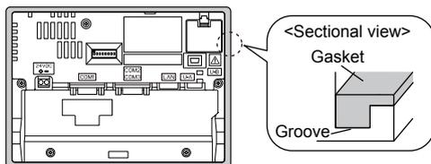
3. Install the TS1000 Smart series unit to the mounting panel and tighten the four fixtures supplied with TS1000 Smart series.
