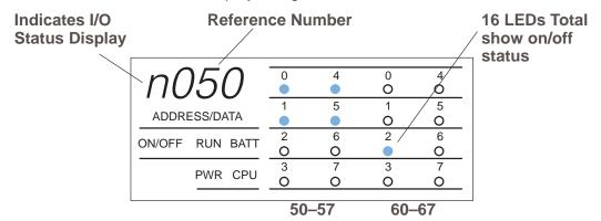
Use the following keystrokes to monitor discrete points. To select a different data type, use the corresponding reference number instead of the one shown. The DL305 memory map is included in Appendix A. This will help you determine the appropriate ranges for the various data types.
