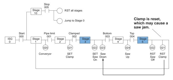
Obviously, there are times when it's perfectly OK to force a program stage on or off. The following example shows the keystrokes required to force an stage.
