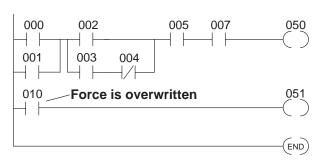
Logic is solved. Point 010, even though previously forced on, is turned off. Points 050 and 051 are turned off since conditions are not met.
