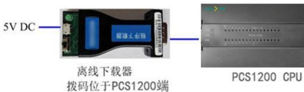
Figure 3 The connection mode of the program downloader SC010 to PCS1200 programmable logic controller
