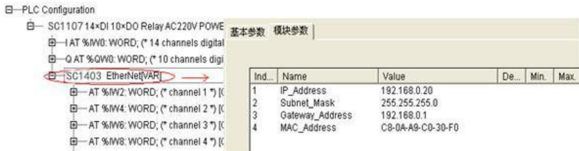
Figure 2 SC1403 configuration diagram
