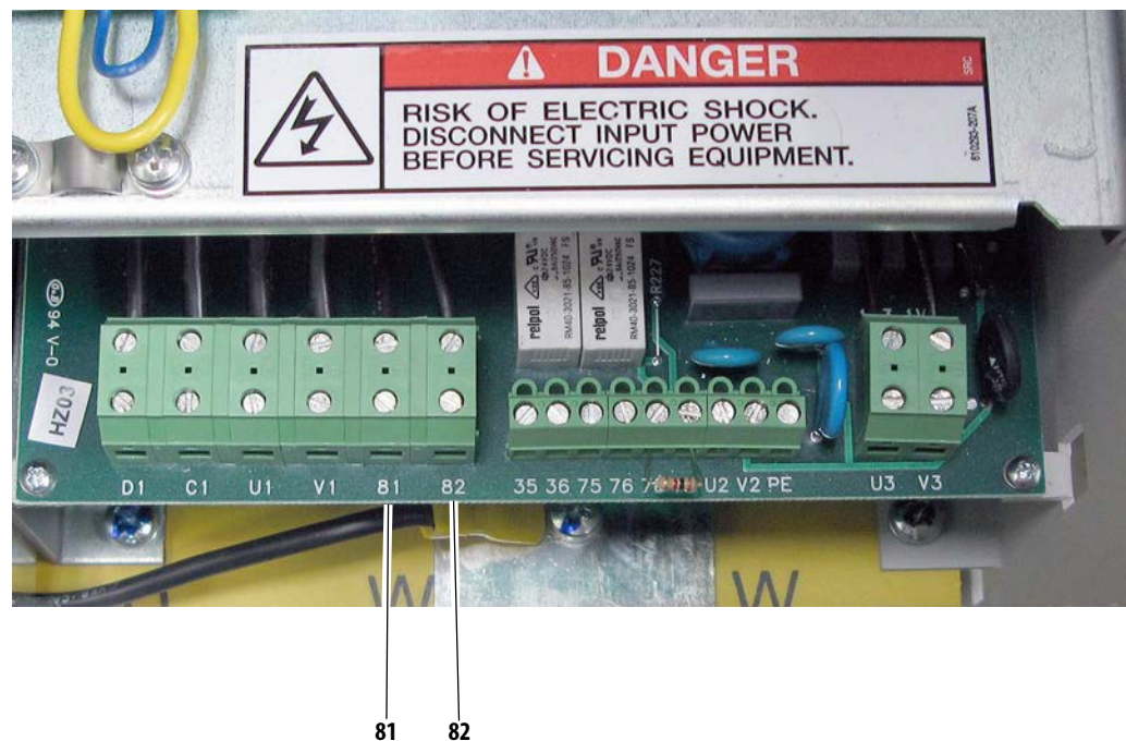
Figure 52 - 230V/460V AC Input Frame C Internal Armature Fuse Signal Terminal Block Location
