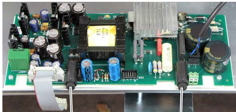
Figure 79 - Frame C Switching Power Supply Circuit Board Fuse Location
